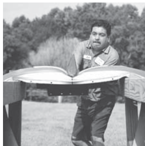
We simulated the effects of a collision by smashing bumpers with a sledgehammer. The Prime Time performed just as well as the 2K urethane in this test.
