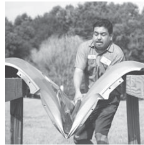
We simulated the effects of a collision by smashing bumpers with a sledgehammer. The Prime Time performed just as well as the 2K urethane in this test.
